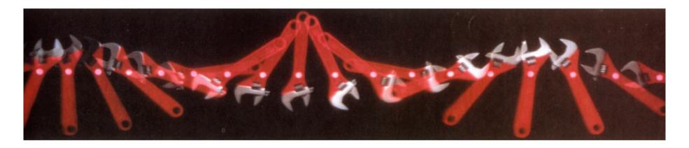
At equilibrium, a body free to rotate will hang so its CM is vertically under the suspension point
