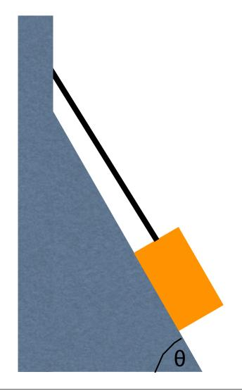
A box is held in position by a cable along a smooth slope, as shown.
