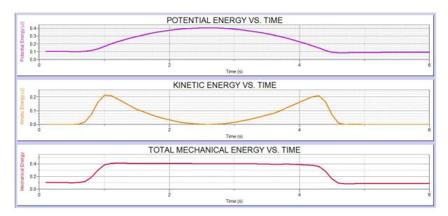
Note that the potential energy is not zero before and after the push. This is simply because, contrary to what it says is the reference level for zero potential energy on the sheet (the height at which the cart is released), in the demo it has actually been defined to be zero at the height of the motion detector, which is a little lower.
