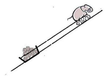
An elephant drags a tray of logs of total weight 10000 N up a uniform slope. The slope is 20 m in length and is inclined at an angle of 30° to the horizontal. The value of the coefficient of kinetic (sliding) friction between the tray of logs and the slope is 0.50. The elephant walks at a constant speed.
