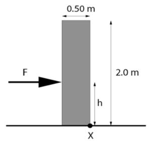
If the block is pushed too near to the top, it will tip over instead of sliding. It will try to rotate about the front corner of the block (labelled X in the diagram).
