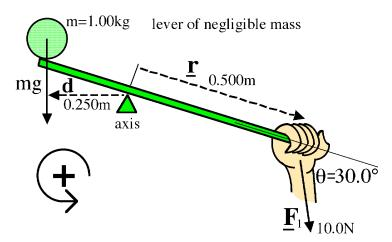
torque 1;  $\underline{\tau}_1 = -rF_1 \sin\theta = -0.5 \times 10 \times \sin 30 = -2.50 \text{ Nm}$ torque 2;  $\underline{\tau}_2 = +mgd = 1 \times 9.8 \times 0.25 = +2.45 \text{ Nm}$
