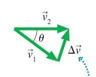
During this motion, the velocity changes direction; the difference vector points toward the center of the circle.
