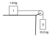
Two weights are attached to a frictionless, massless pulley. (a) Find the magnitude of acceleration of the blocks (b) Find the tension in the string.
