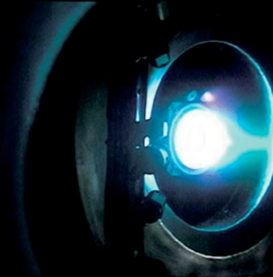
The SMART-I ion engine being test fired.
