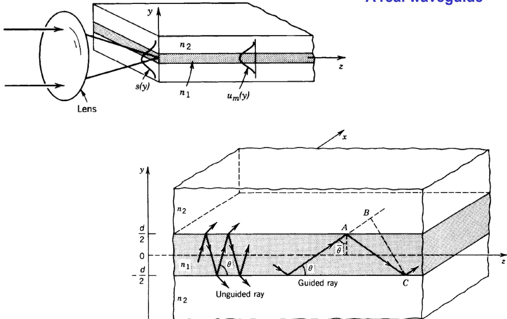
**Figure 7.2-1** Planar dielectric waveguide. Rays making an angle  $\theta < \bar{\theta}_c = \cos^{-1}(n_2/n_1)$  are guided by total internal reflection.
