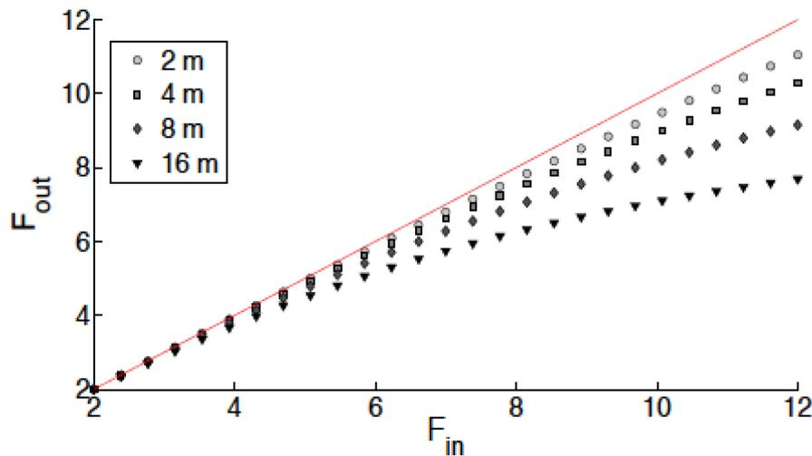
Analytically derived from formulae by Gloge (1971) and Snyder & Love (1983) where light in any give mode (angle to fibre axis) gets scattered. Since higher modes have more volume, light tends to scatter from low to high modes, until natural NA of fibre is filled.
