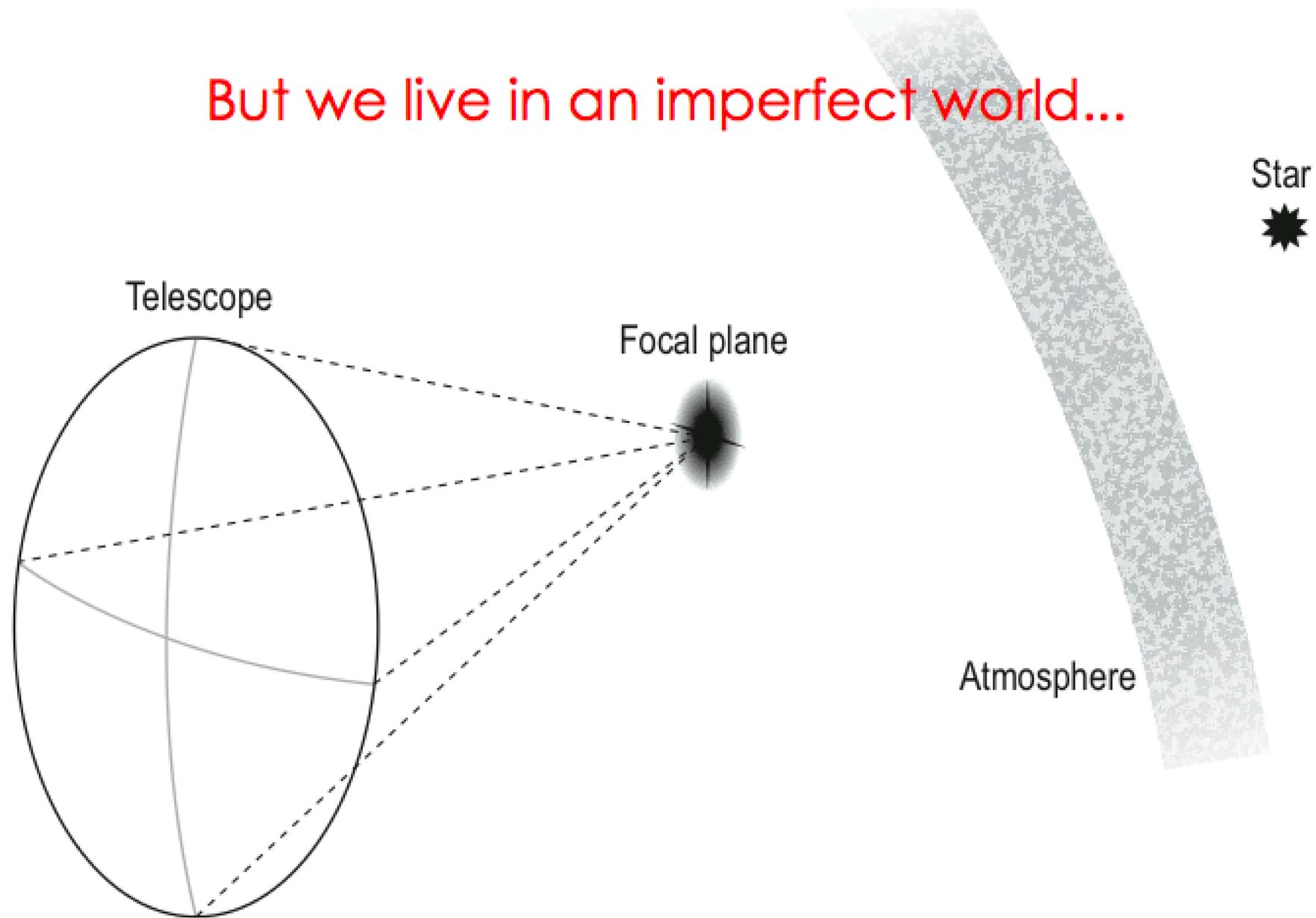
Telescope PSF is imperfect gaussian such that  $M \gg 0$
