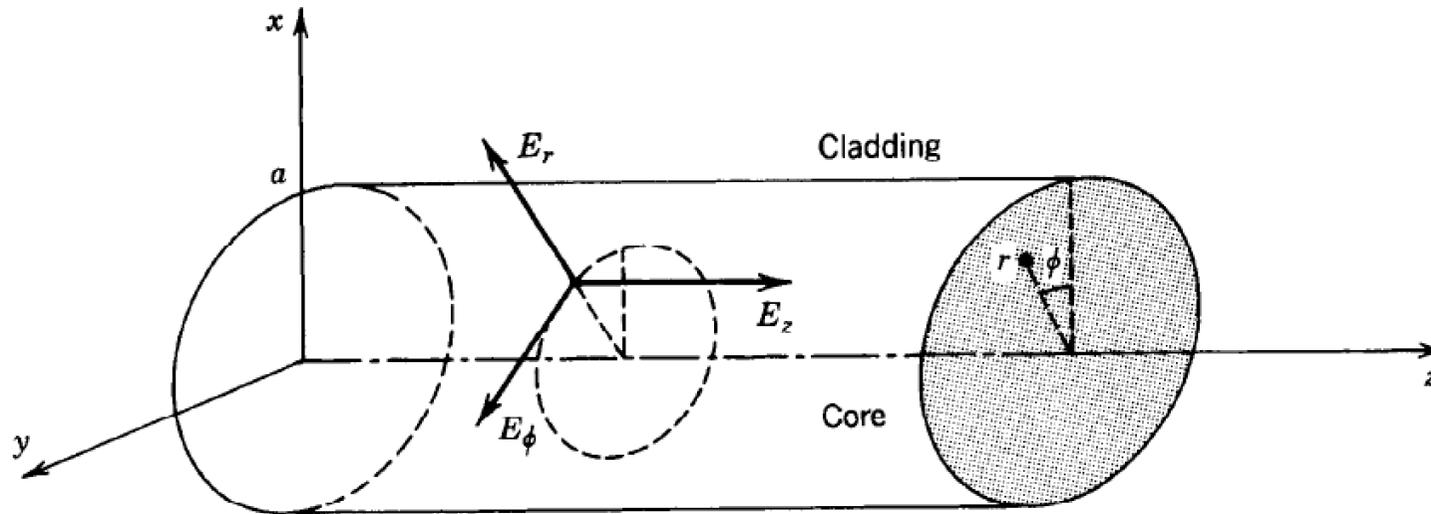
**Figure 8.1-4** Cylindrical coordinate system.
