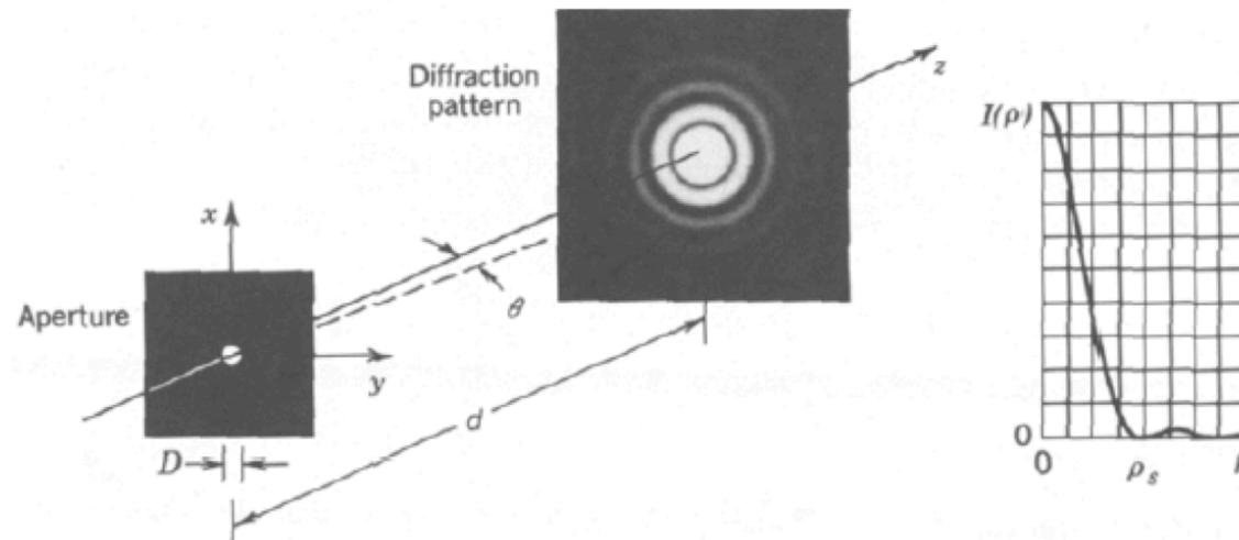
**Figure 4.3-4** The Fraunhofer diffraction pattern from a circular aperture produces the Airy pattern with the radius of the central disk subtending an angle  $\theta = 1.22\lambda/D$ .
