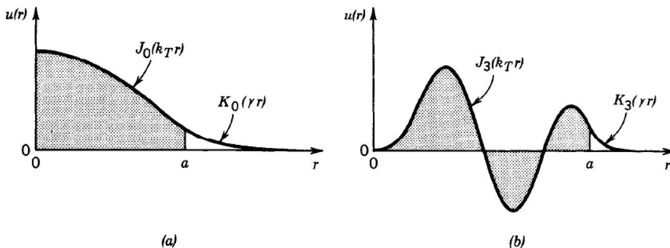
**Figure 8.1-5** Examples of the radial distribution  $u(r)$  given by (8.1-9) for (a)  $l = 0$  and (b)  $l = 3$ . The shaded areas represent the fiber core and the unshaded areas the cladding. The
