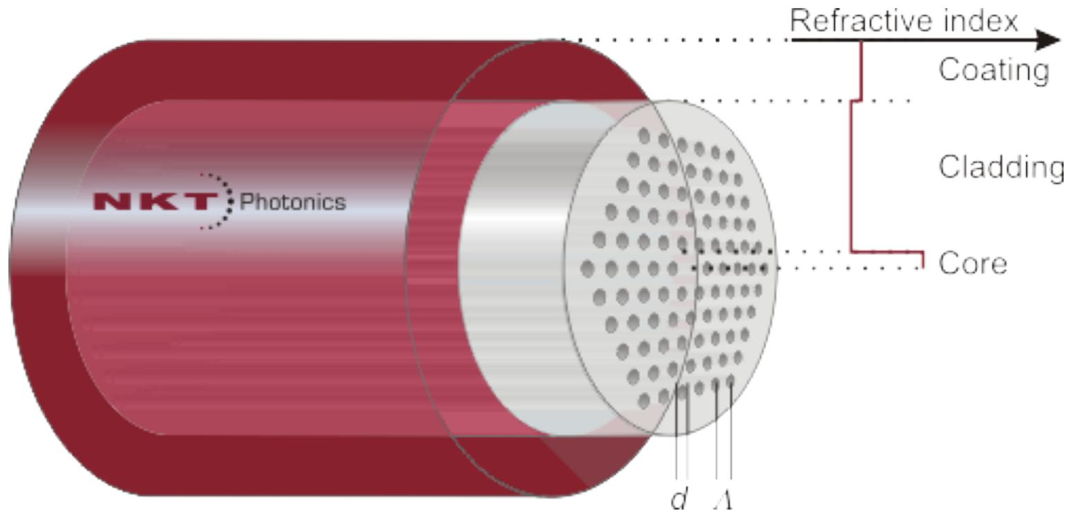
The guiding properties are determined by the hole sizes, separations and patterns. Invented by our colleague Phillip Russell in 1996. Sometimes there is a large central hole, or a central region devoid of holes, etc. There are very many permutations, active R&D.
