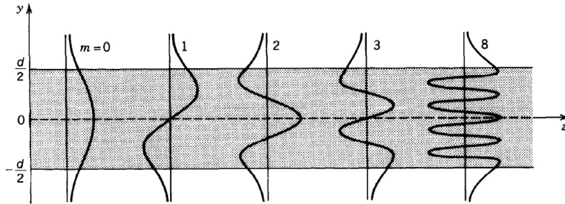
**Figure 7.2-5** Field distributions for TE guided modes in a dielectric waveguide. These results should be compared with those shown in Fig. 7.1-4 for the planar-mirror waveguide.
