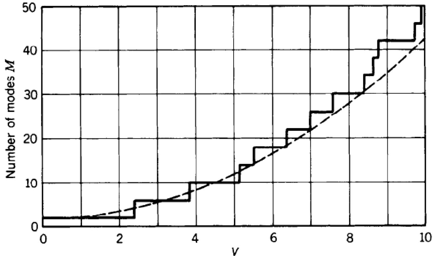
**Figure 8.1-8** Total number of modes  $M$  versus the fiber parameter  $V = 2\pi(a/\lambda_o)NA$ . Included in the count are two helical polarities for each mode with  $l > 0$  and two polarizations per mode. For  $V < 2.405$ , there is only one mode, the fundamental  $LP_{01}$  mode with two polarizations. The dashed curve is the relation  $M = 4V^2/\pi^2 + 2$ , which provides an approximate formula for the number of modes when  $V \gg 1$ .
