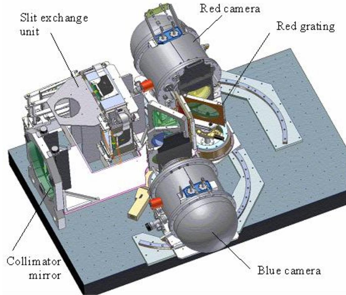
Figure 1. Physical layout of AAOmega, layout, showing the red camera in high dispersion mode, and blue camera in low dispersion mode.
