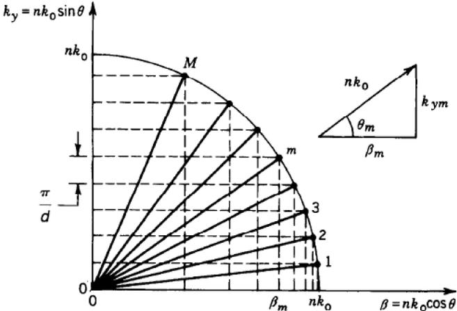
**Figure 7.1-3** The bounce angles  $\theta_m$  and the wavevector components of the modes of a planar-mirror waveguide (indicated by dots). The transverse components  $k_{ym} = k \sin \theta_m$  are spaced uniformly at multiples of  $\pi/d$ , but the bounce angles  $\theta_m$  and the propagation constants  $\beta_m$  are not equally spaced. Mode  $m = 1$  has the smallest bounce angle and the largest propagation constant.
