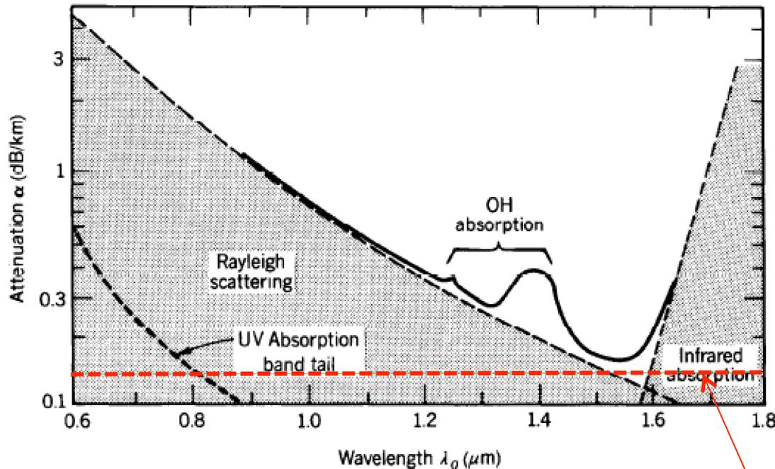
**Figure 8.3-2** Dependence of the attenuation coefficient  $\alpha$  of silica glass on the wavelength  $\lambda_0$ . There is a local minimum at 1.3  $\mu\text{m}$  ( $\alpha \approx 0.3$  dB/km) and an absolute minimum at 1.55  $\mu\text{m}$  ( $\alpha \approx 0.16$  dB/km).
