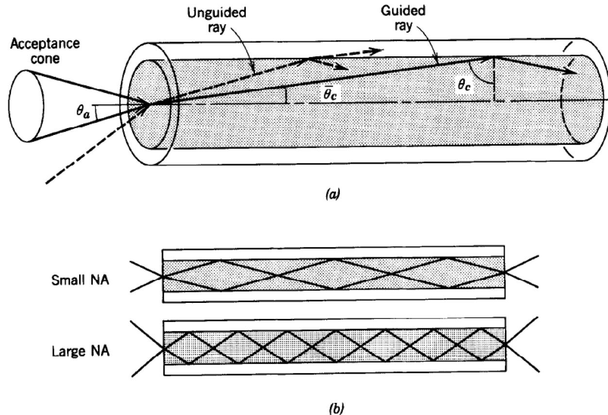
**Figure 8.1-3** (a) The acceptance angle  $\theta_a$  of a fiber. Rays within the acceptance cone are guided by total internal reflection. The numerical aperture  $NA = \sin \theta_a$ . (b) The light-gathering capacity of a large NA fiber is greater than that of a small NA fiber. The angles  $\theta_a$  and  $\bar{\theta}_c$  are typically quite small; they are exaggerated here for clarity.
