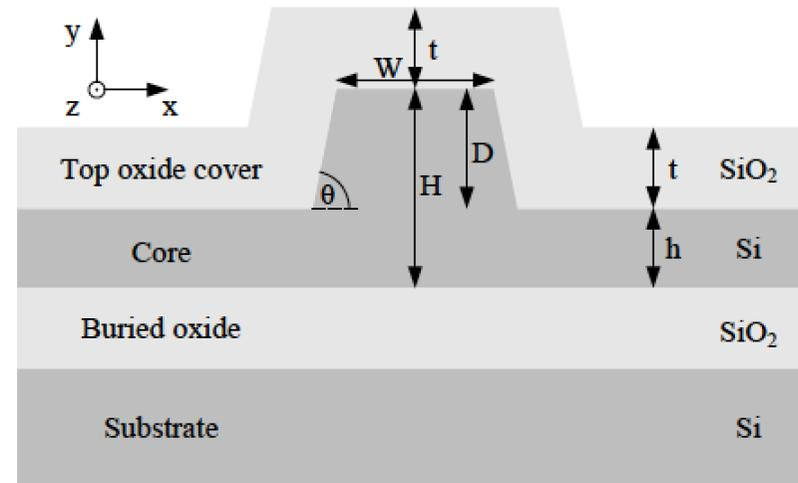
Rib waveguide ( $H=400$  nm to several microns; 0.1 dB/cm loss)
