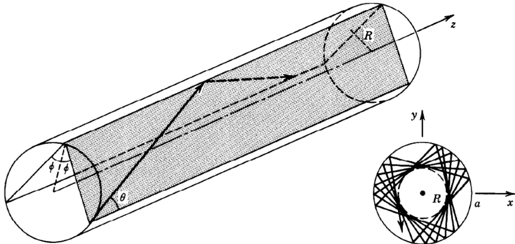
The ray analogy is of limited use - much of the energy moves in azimuth, i.e. missing the optical axis. Fibres are fantastic at scrambling information in azimuth; scrambling in radius is far harder, hence the **scrambling problem** you may have heard about in the context of planet hunting spectroscopy. (Polarization-maintaining fibres do exist.)
