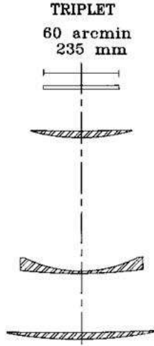
Figure 5. Schematic of AAT prime focus triplet corrector.
