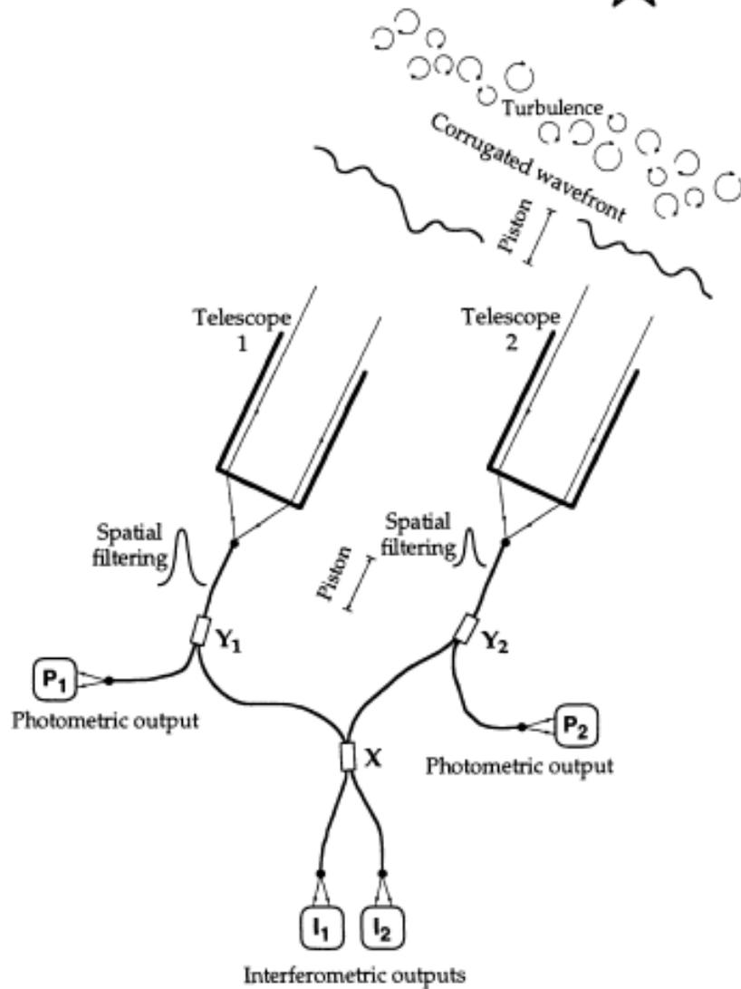
Figure 1. Conceptual design of a stellar fiber interferometer.
