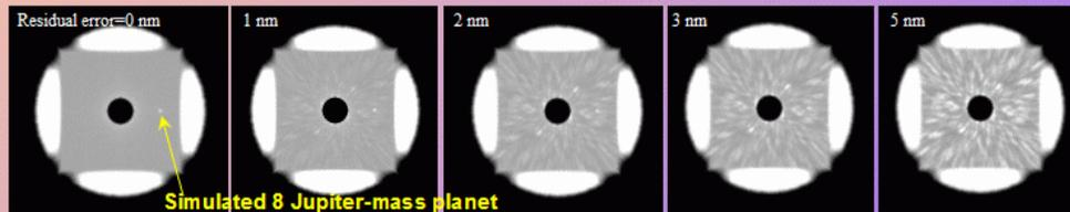
The Extreme Adaptive Optics Planet Imager will require very low static wavefront error within the frequency range the deformable mirror can correct for. The simulations above demonstrate why. At just one nm of residual error scattered light is visible and at 3 nm the planet is very difficult to detect. The XAOPI error budget calls for errors at the 2 nm level. In the first phase of our testbed we measure static errors and in the next phase we will use a deformable mirror to correct them.
