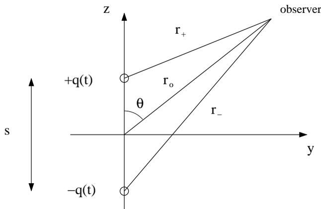
Figure 3.2: Dipole radiator.
